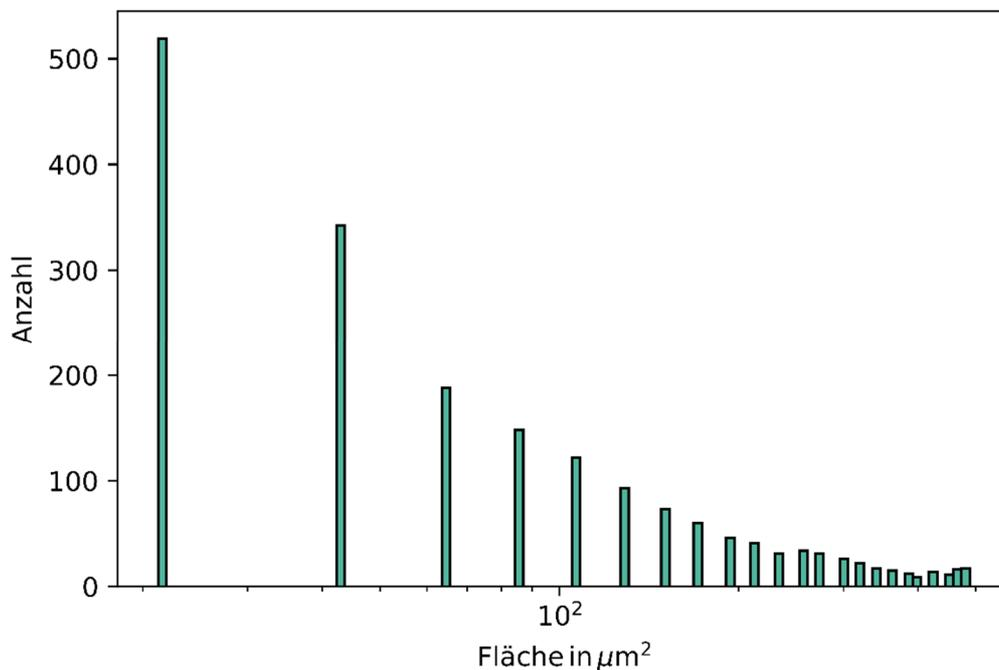
Figure 10: Section of a histogram of the pore area distribution in the micrograph in semi-logarithmic representation from 0 to  $500\mu\text{m}^2$ . Due to the discrete number of pixels, the pore size and area cannot be represented continuously.
