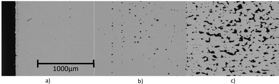
Figure 4. Detailed micrographs of specimens with a) edge porosity, b) gas pores and c) brittle pores.
