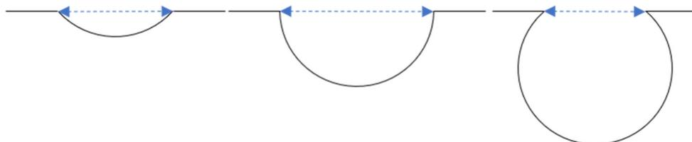
*Figure 2: Determination of the pore size via the visible diameter on the ground surface.*
