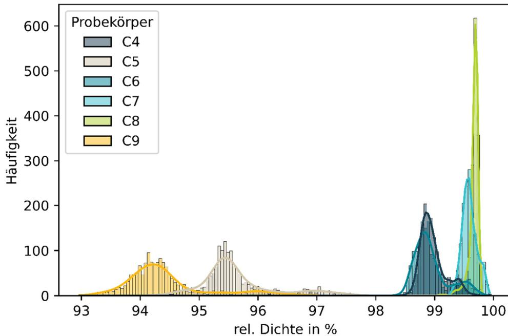
Figure 6 Histogram of the relative density of the CT scans for specimen C4-C9.
