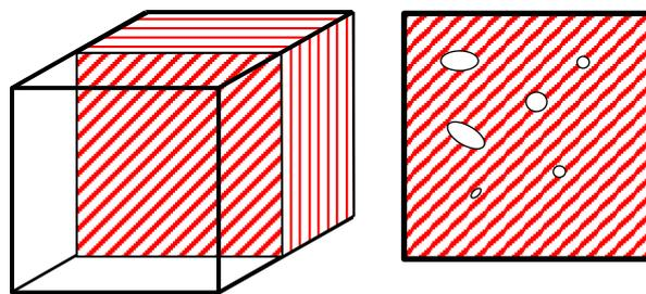
*Figure 1. Schematic representation of a cross-section and the resulting micrograph with defects.*
