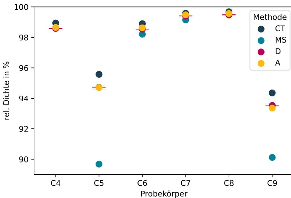
Figure 8: Relative percent density for specimens C4-C9 with paint-of-fusion defects.
