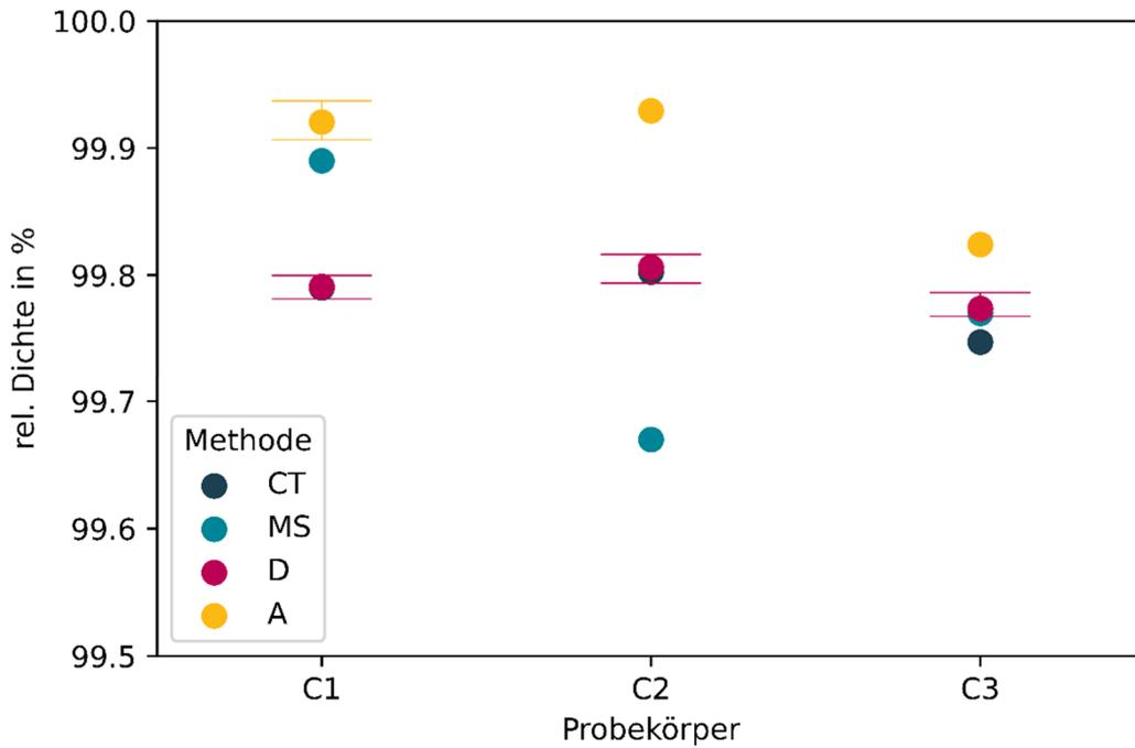
Figure 7: Relative density in percent for the reference specimens C1-C3.
