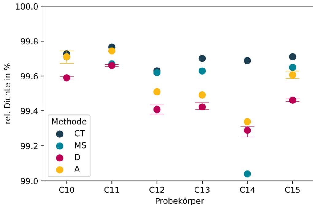
Figure 9: Relative density in percent for the test specimens C10-C15 with gas pores.
