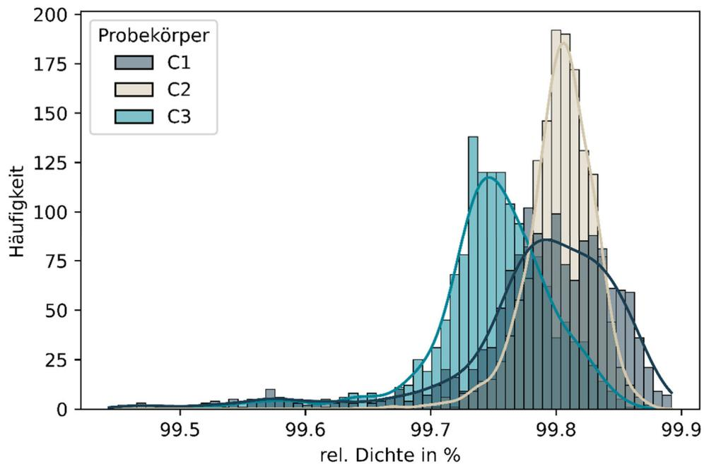
Figure 5 Histogram of the relative density of the CT scans for specimen C1-C3.
